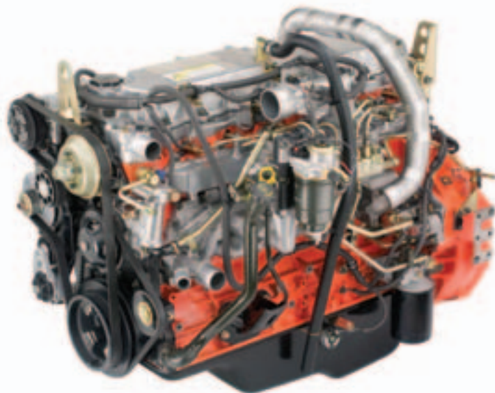
This 7.8-liter inline 6-cylinder is the first diesel engine produced by the joint venture between GM and Isuzu. The 7800 was introduced in 2000 medium-duty trucks, and comes in 200-hp/520-ft-lb or 275-hp/860-ft-lb versions. (Photo courtesy of General Motors)
