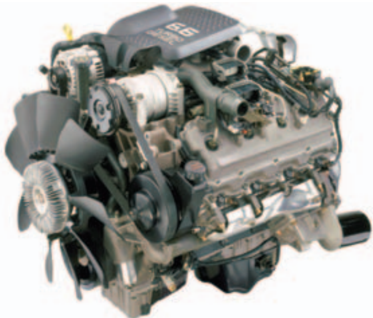
For the 2004 model year, the LB7 Duramax 6600 6.6L diesel V-8 was rated at 300 hp at 3,100 rpm and 520 ft-lbs of torque at 1,800 rpm. The LB7 came in 2001 to 2004 GM light heavy-duty trucks. It did not use EGR but did have catalytic converters where required. (Photo courtesy of General Motors)
