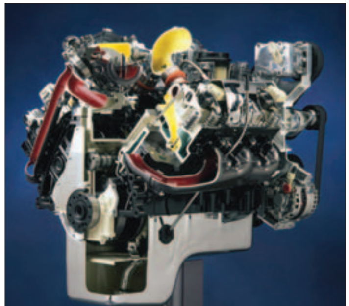
This 7.3-liter cutaway model shows the airflow path on the hot and cold sides of the turbo system. Notice the intake port profile. It looks like a high-flowing port on a performance engine. (Photo courtesy of Ford)
