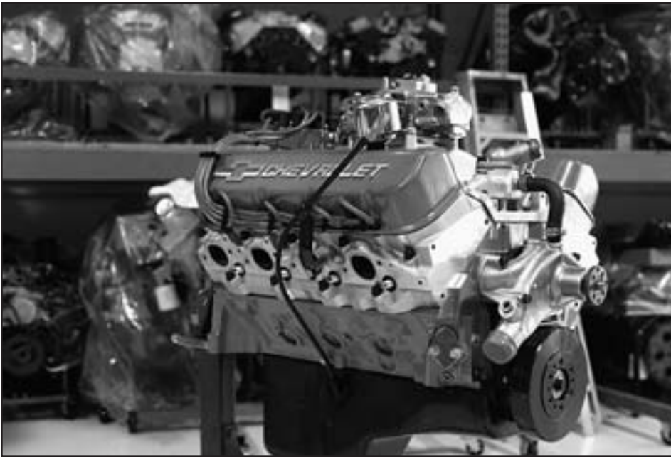
F.A.S.T. makes ECUs to handle nearly every type of engine available. A very popular application would be something like this big-block Chevrolet engine. F.A.S.T. can fire the eight injectors in bank-to-bank or sequential mode.
