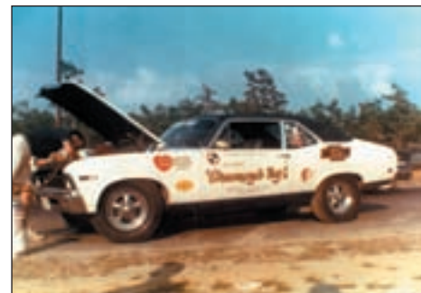
Bill Jenkins campaigned a couple of big-block Chevrolets in 1968, including Grumpy's Toy V, a Nova coupe with a 375-horse 396. Racing in SS/D, the Nova was ready to step up if the SS/C Camaro would get beaten. Note the tall but narrow Stahl tires on the front, used to gain a fraction of a second in the starter beams. (Jack Bleil)
