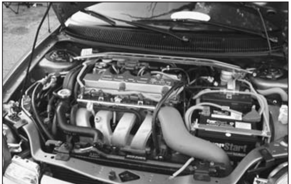
Installing an aftermarket intake system is probably the best bang for the buck for a Neon 2.0-liter powerplant. The potential for gain is even higher for a 2001-'04 R/T and a 2001-'02 ACR. This is an Iceman intake on a first-generation Neon. (Photo courtesy Patrick O'Hara)
