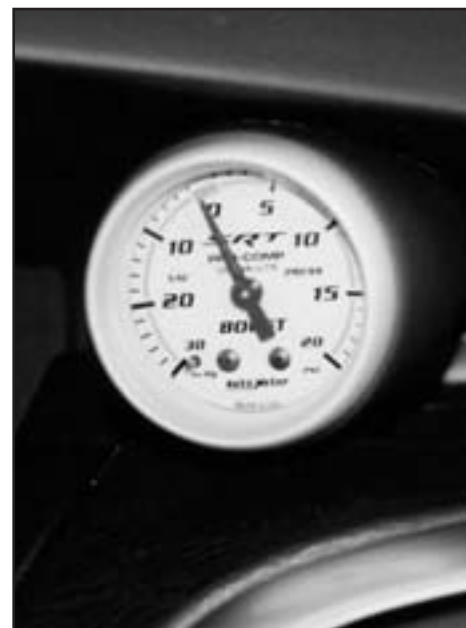
The SRT-4 gauge array is both functional and informative. All turbo engines should have a boost gauge, and the SRT-4 comes with one from the factory (right). Besides showing you how much boost you’re making, boost gauges also show you the boost you don’t have (when something breaks!).
