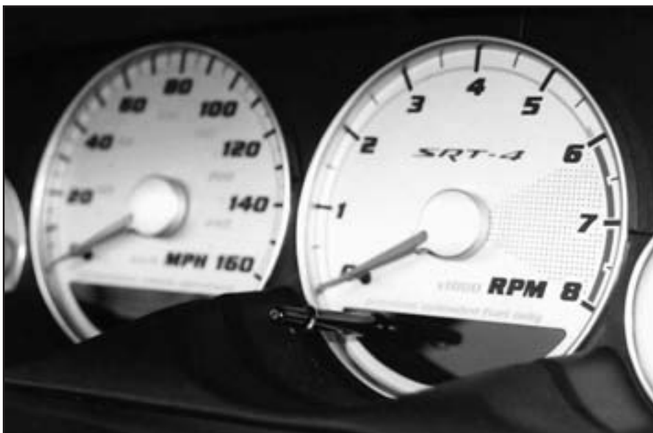
The SRT-4 gauge array is both functional and informative. All turbo engines should have a boost gauge, and the SRT-4 comes with one from the factory (right). Besides showing you how much boost you’re making, boost gauges also show you the boost you don’t have (when something breaks!).
