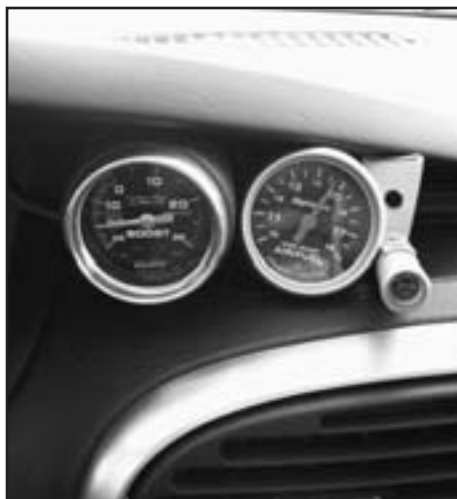
The owner of this SRT-4 has added some essential gauges. From left to right: a boost gauge, a wide-band air/fuel ratio gauge, and a shift light. (Photo courtesy Chris Malluege)
