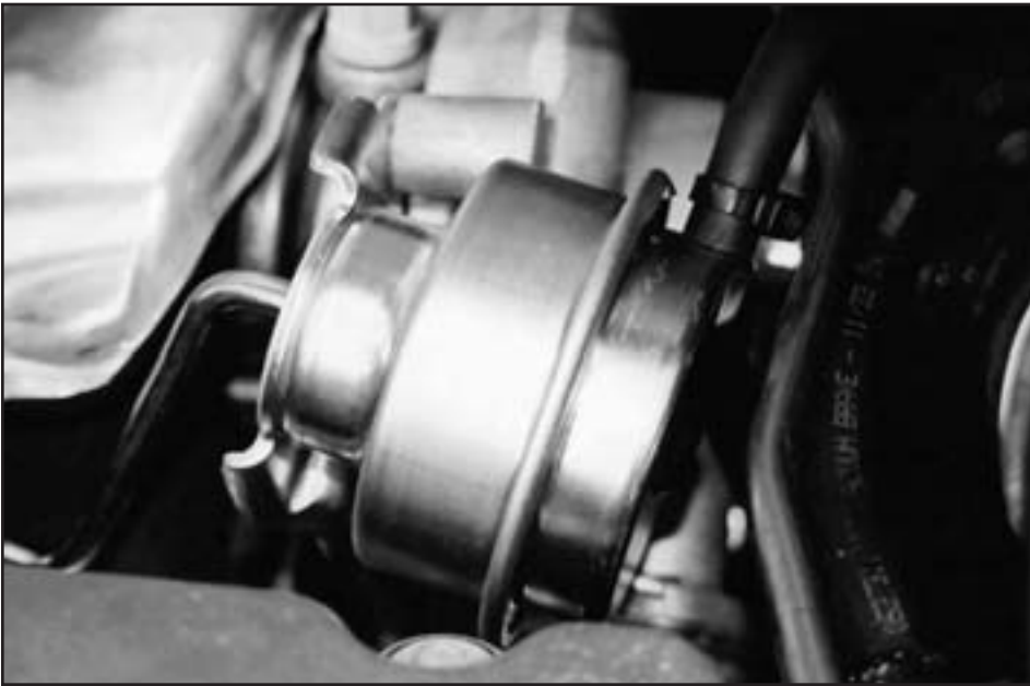
Mounting a wastegate can be a bit of a challenge. You have to make sure that it's adjusted properly so that the valve is fully closed (no leakage) when the system is under boost.
