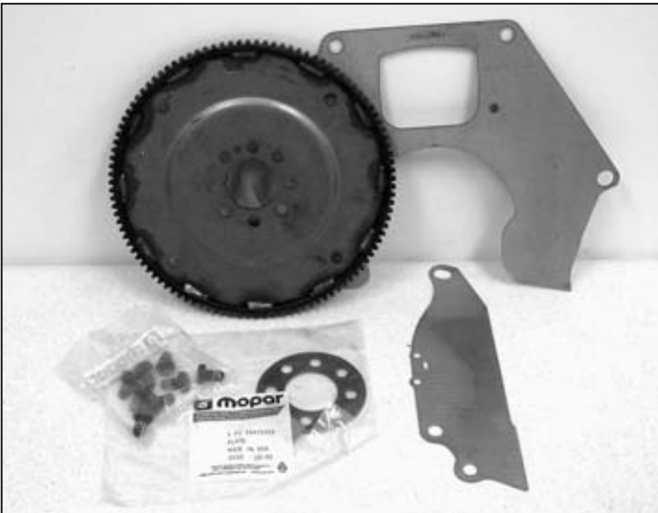
Mopar Performance Parts offers a kit to help you install a modular clutch assembly in place of your traditional clutch and flywheel assembly. Once you install a modular clutch with this kit, installing another modular clutch is as simple as swapping it in.
