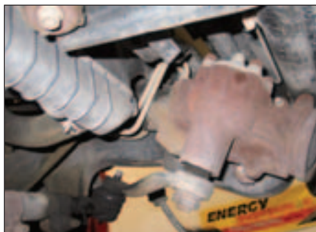
Power steering became standard equipment on the Wrangler TJ in 2000. Jeep Wranglers used a recirculating ball steering gear made by Saginaw/Delphi from '97 to 2002.
