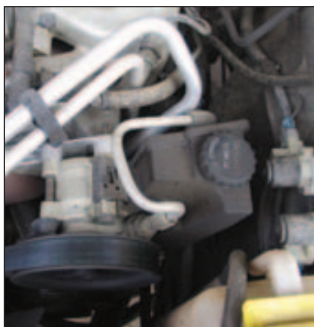
The stock 4.0L power steering pump, known as a TC-type pump, uses an external reservoir that clips to the pump body.
