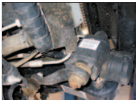
From '03 to '06 TJs came equipped with a steering gear made by ZF Gear. A few differences are apparent, including the overall shape and the bolt pattern to the frame.
